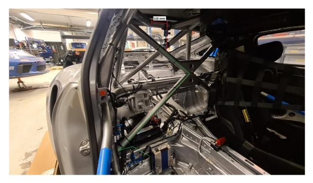
Rear facing camera mounting position and wiring harness routing:
